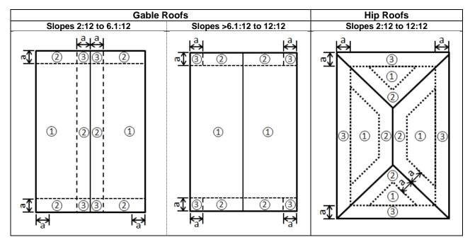
Dimension "a" shall be 10% of the least horizontal dimension or (0.4 x *Mean Roof Height*), whichever is smaller, but not less than either 4% of the least horizontal dimension or 3ft.
